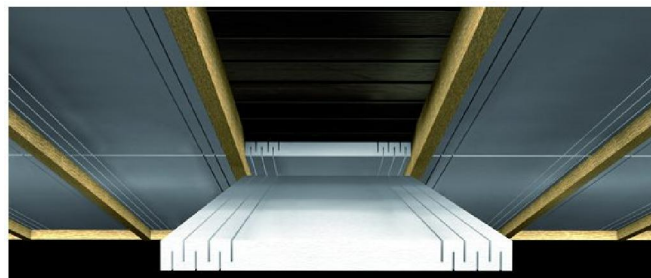
Under floor polystyrene
