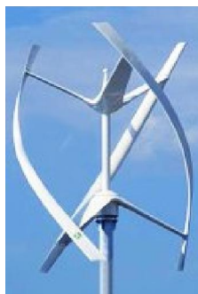
Vertical Axis Wind Turbine (VAWT)
